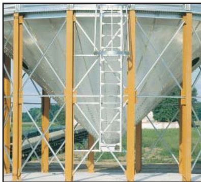
45 degree hopper slope
